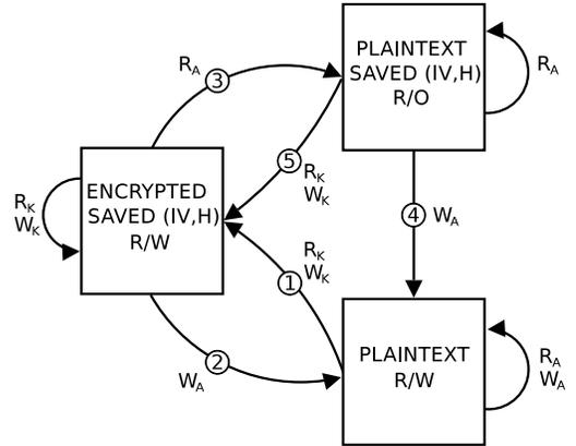
**Figure 1. Basic Cloaking Protocol.** State transition diagram for maintaining the secrecy and integrity of a single cloaked page. Application reads  $R_A$  and writes  $W_A$  manipulate plaintext page contents, while kernel reads  $R_K$  and writes  $W_K$  use an encrypted version of the page. A secure hash  $H$  is computed and stored immediately after page encryption, and verified immediately prior to page decryption.
