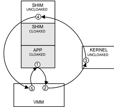
Figure 3. Control Flow for Handling Faults and Interrupts
