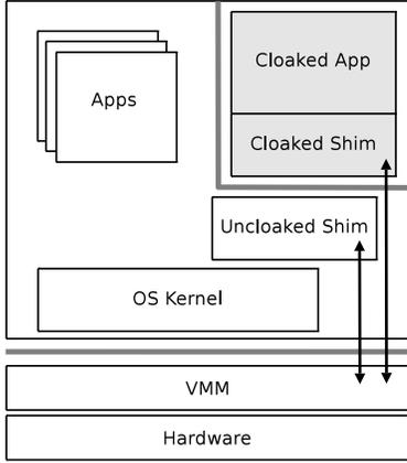
**Figure 2. Overshadow Architecture.** The VMM enforces two virtualization barriers (gray lines). One isolates the guest from the host, and the other cryptographically isolates cloaked applications from the guest OS. The shim cooperates with the VMM to interpose on all control flow between the cloaked application and OS.
