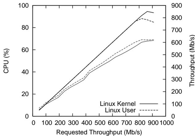
Figure 4: UDP echo throughput and CPU utilisation
